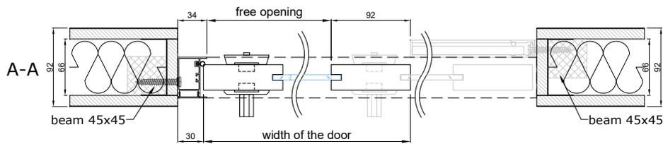
CONNECTION WITH WALL (WITH LOCKING AND PULL HANDLES)
