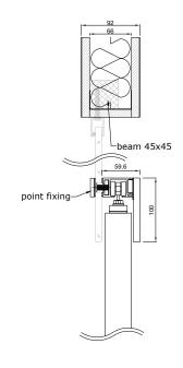
$\circ$  - seal, EPDM-50Dha\_5mm\_BLACK
