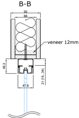
CONNECTION WITH CEILING USING E-PROFILE
