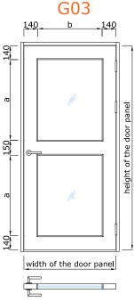
a = (height of the door panel - 430mm) / 2b = width of the door panel - 280mm
