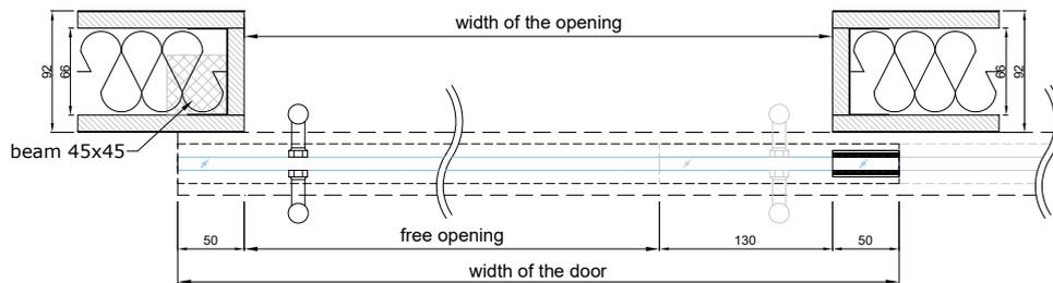
CONNECTION WITH WALL (WITH STRIKER PROFILE AND PULL HANDLES)
