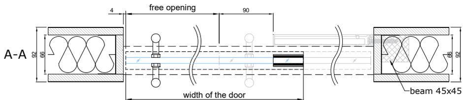
CONNECTION WITH WALL (WITH STRIKER PROFILE AND PULL HANDLES)
